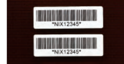
Polyimide STATINIX Top: Pre-reflow Bottom: Post-reflow; No change
